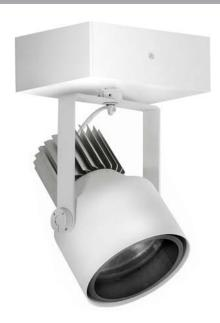
Artima/5 HI O LH-OBM is a surface mounted accent light powered by two sets of Citizen chip-on-board LED modules: one set providing a CRI of 97 within 2-step MacAdam ellipses; and one set providing a CRI of 80 within 3-step MacAdam ellipses. See tables on the reverse for wattages and efficiacies.
