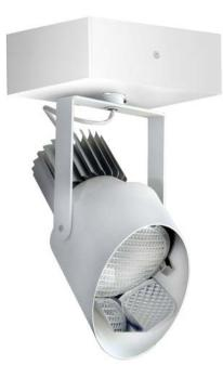
Artima/5 HI W-OBM is a surface mounted wallwasher powered by two sets of Citizen chip-on-board LED modules: one set providing a CRI of 97 within 2-step MacAdam ellipses; and one set providing a CRI of 80 within 3-step MacAdam ellipses. See tables below for wattages and efficiacies.
