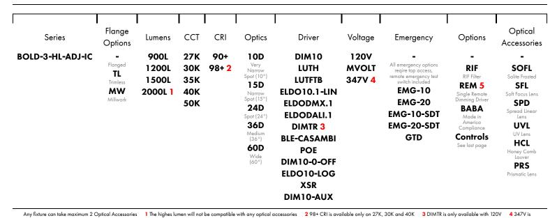
only available with DIM10 5 Remote mount Maximum distance from light fixture to remote power supply is 100' using 14 gauge wire, 50' using 16 gauge wire
