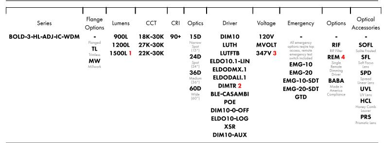
Any fixture can take maximum 2 Optical Accessories 1 The highes lumen will not be compatible with any optical accessories Maximum distance from light fixture to remote power supply is 100' using 14 gauge wire, 50' using 16 gauge wire
