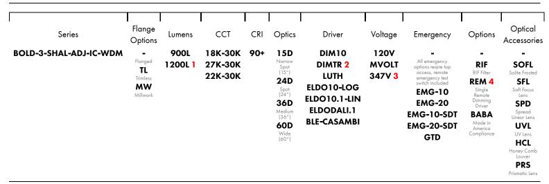
Any fixture can take maximum 2 Optical Accessories 1 The highes lumen will not be compatible with any optical accessories 2 DIMTR is only available with 120V 3 347V is only available with DIM10 4 Remote mount Maximum distance from light fixture to remote power supply is 100' using 14 gauge wire, 50' using 16 gauge wire
