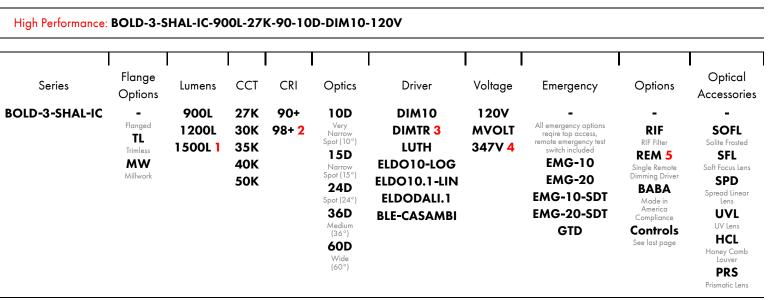
Any fixture can take maximum 2 Optical Accessories 1 The highes lumen will not be compatible with any optical accessories 2 98+ CRI is available only on 27K, 30K and 40K 3 DIMTR is only available with 120V 4 347V is only available with DIM10 5 Remote mount Maximum distance from light fixture to remote power supply is 100' using 14 gauge wire, 50' using 16 gauge wire
