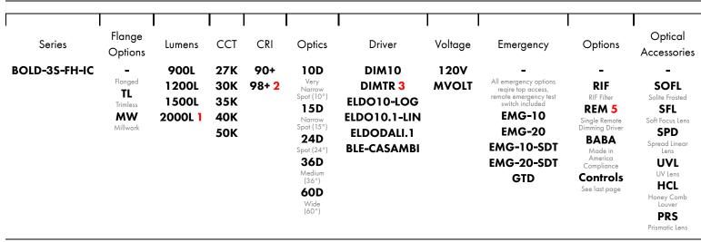
Any fixture can take maximum 2 Optical Accessories 1 The highes lumen will not be compatible with any optical accessories 2 98 + CRI is available only on 27K, 30K and 40K 3 DIMTR is only available with 120V 4 347V is only available with DIM10 5 Remote mount Maximum distance from light fixture to remote power supply is 100' using 14 gauge wire, 50' using 16 gauge wire
