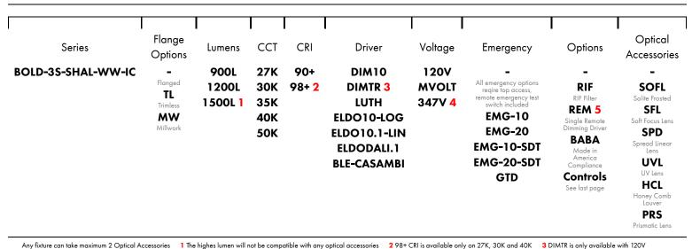
Any tixture can take maximum 2 Optical Accessories 1 the highes lumen will not be compatible with any optical accessories 2 98+ CRI is available only on 27K, 30K and 40K 3 DIMTR is only available with 120V 4 437V is only available with DIMTO 5 Remote mount Maximum distance from light fixture to remote power supply is 100' using 14 gauge wire, 50' using 16 gauge wire
