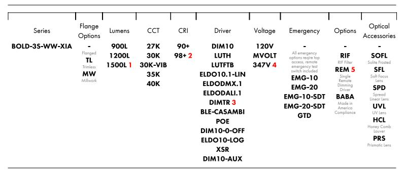
Any fixture can take maximum 2 Optical Accessories 1 The highes lumen will not be compatible with any optical accessories 2 95+ CRI is not available on 50K 3 DIMTR is only available with 120V 4 347V is only available with DIM10 5 Remote mount Maximum distance from light fixture to remote power supply is 100' using 14 gauge wire, 50' using 16 gauge wire
