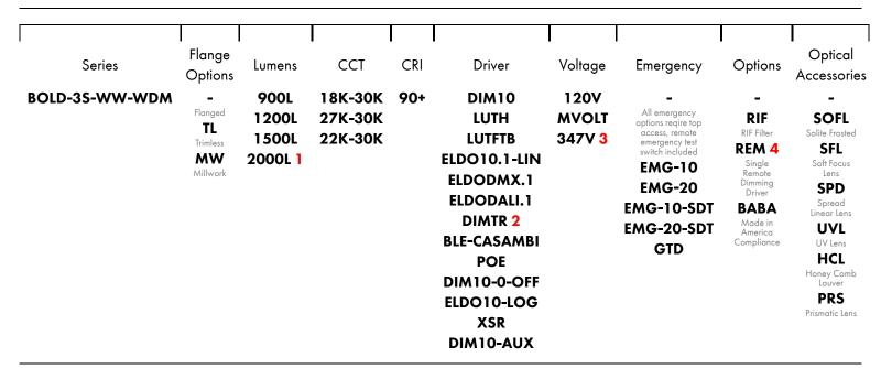
Any fixture can take maximum 2 Optical Accessories 1 The highes lumen will not be compatible with any optical accessories 2 DIMTR is only available with 120V 3 347V is only available with DIM10 4 Remote mount Maximum distance from light fixture to remote power supply is 100' using 14 gauge wire, 50' using 16 gauge wire
