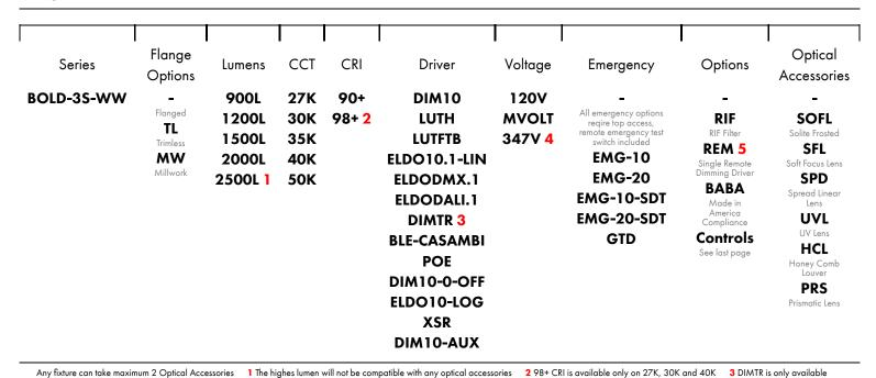
5 Remote mount Maximum distance from light fixture to remote power supply is 100' using 14 gauge wire, 50' using 16 gauge wire
