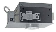
Luminaire is listed for Damp Location. Fixture is prewired with an insulation detecting thermal protector. Luminaire approved for eight #12 wire 90° C branch circuit pull through wiring and is suitable for use in a fire rated ceiling. Removal of the external reflector allows access to the LED module and junction box.
