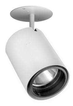
IDM Maxima CZS O LH-OBM is a surface mounted open-aperture accent light capable of 9° to 40° beam spreads. Fixture is powered by Citizen chip-on-board LED's providing either a CRI of 97 within 2-step MacAdam ellipses or a CRI of 80 within 3-step MacAdam ellipses. See tables on reverse for wattages and efficacies.
