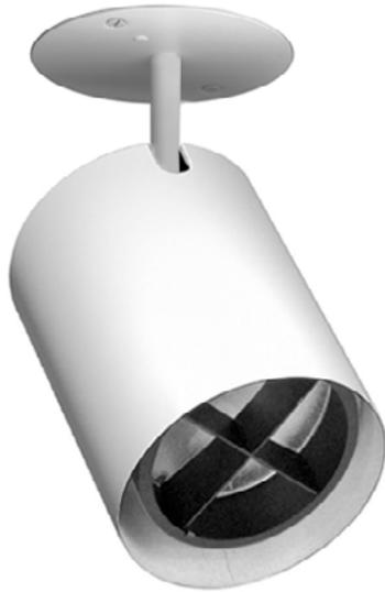
IDM Maxima XTM O-OBM is a surface mounted accent light powered by one of two Xicato LED modules, all of which are distinguished by extraordinary color consistency (within 1x2-step MacAdam ellipse). See tables on the reverse for wattages and efficacies.
