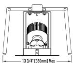
Luminaire is listed for Damp Location, RoHA compliant and prewired with a thermal protector. Removal of the reflector allows access to the LED array, driver and junction box.
