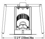
Luminaire is . Issted for Damp Location, RoHA compliant and prewired with a thermal protector. Removal of the reflector allows access to the LED array, driver and junction box.
